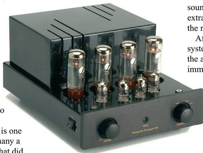
transformers with wide frequency band for extended low and high frequencies. These transformers were developed by Marcel Croese, one of the most renowned audio designers, together with a "known" American transformer-designer. Ventilated ceramic sockets were used for the tubes, and an **Alps** potentiometer for the volume. **Nichicon** and **Real Caps** capacitors and gold-plated binding posts of the WBT type and RCA terminals were used.
