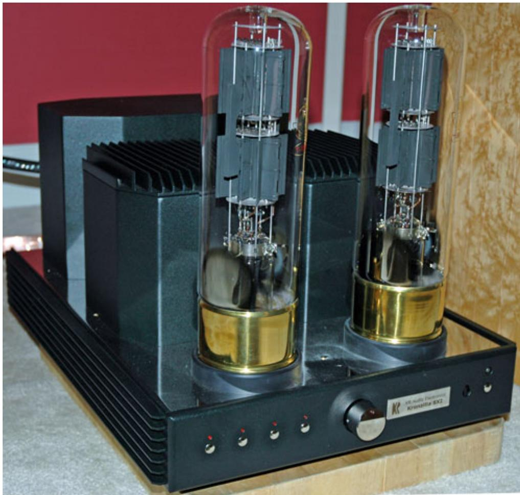
Just 2 tubes need to be fitted to the amplifier, but what tubes they are! 14" tall by 4" in diameter, these are the largest used for audio that I'm aware of. I've heard that they trace their lineage to military radio sets of the 1940s but, according to Eunice Kron, they were developed
