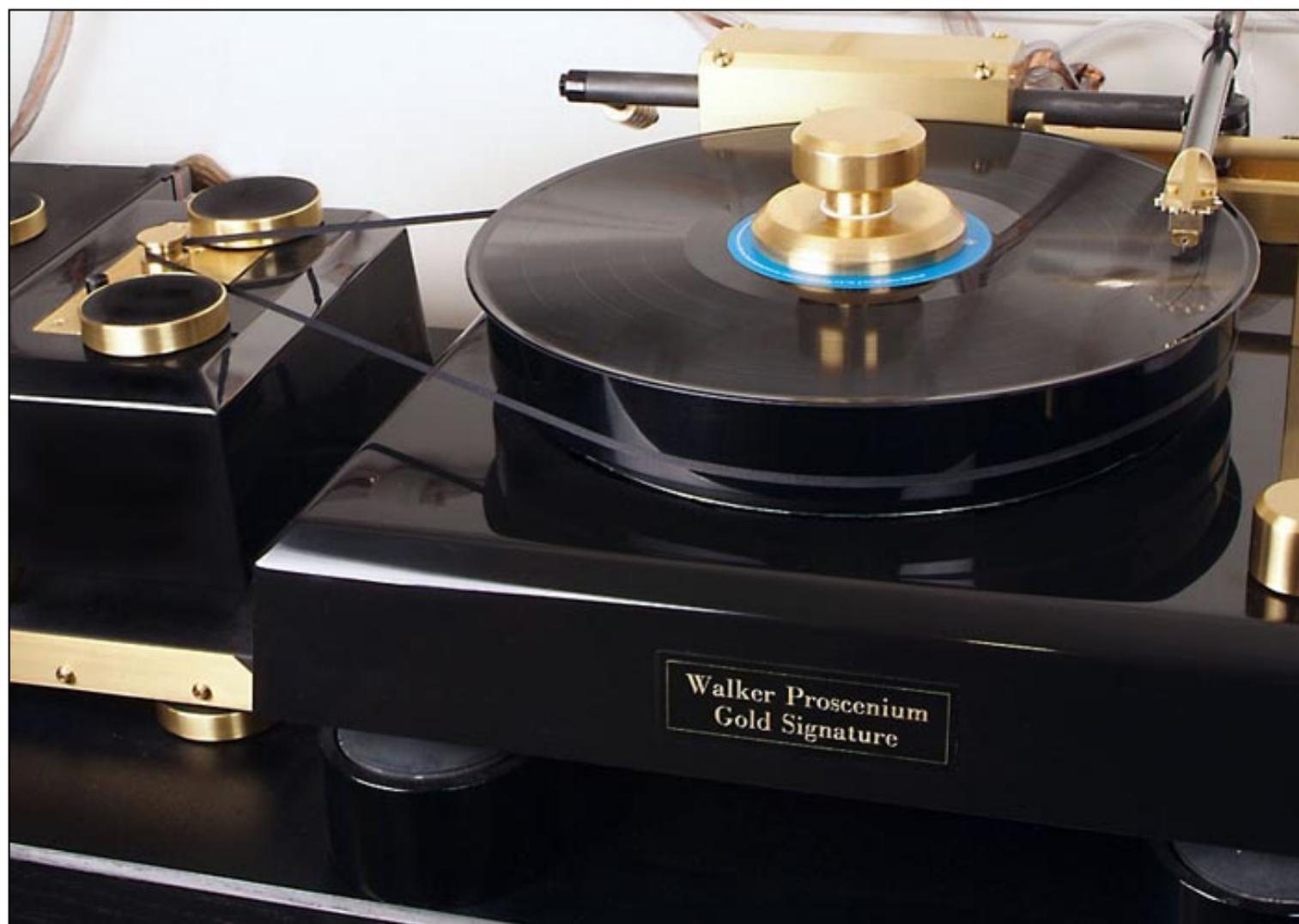
The Goldfinger feeds the Walker Reference phono preamp whose 1K resistive loading provides a good match with most cartridges. The Goldfinger was no exception with its internal resistance at 50  $\Omega$ . A loading of twenty times the internal resistance generally is a good match.
